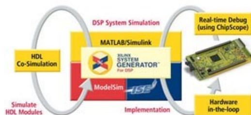
Figure 2. Outline the operation of Xilinx System Generator tool [4].
